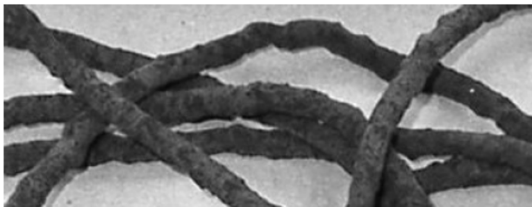
Figure 6.1: Picture of reclaimed EPDM building-profile material after extrusion 12
